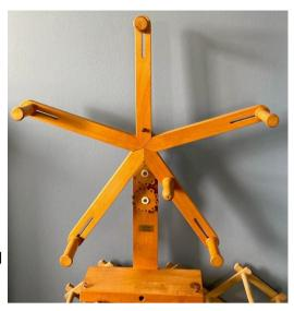
The skein winder also measures the yarn automatically through the dials in the centre so I know all my skeins will be the same in length, and weight if my spinning is consistent. I put skeins on when I am turning them into balls for knitting and crochet and can wind a pirn directly too when weaving
